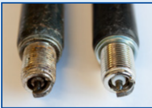
Spark plug after use and after cleaning
