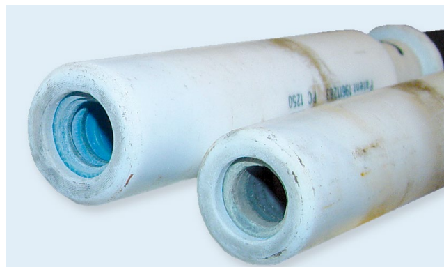
Proper insulation is no longer provided and replacement is necessary for further operation.
